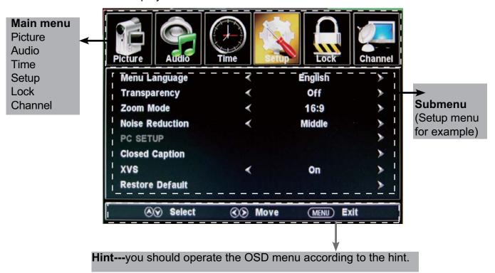
Use < / > button to select the main menu, and press  $\lor$  button to enter the submenu. In the submenu, use  $\land$  /  $\lor$  button to select the function item, press < / > button to adjust/setup, or press > button to enter the submenu.
